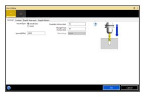
EDGECAM now provides a Gun Drilling cycle. This dedicated interface aims to simplify the information contained in the dialog and provide the same functionality as in the Deep Hole tab of the Hole cycle but with some additional controls.
