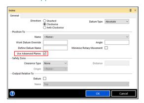
When indexing to a Workplane that would normally require it to be aligned to the machine axes, EDGECAM will leave it in its current orientation and moves and cycles will be relative to that plane.
