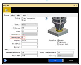
Previously, a stock offset was used to ensure that the Face Mill cycle tool cut over the stock edge but this also meant that the length of cut increased.
