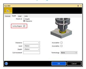
Because Face Milling can recognise the current stock, the cycle can be used to machine the top area of different bosses. However, previously, the cuts had no proper order and the tool could jump around between the different areas causing a lot of unnecessary moves.
