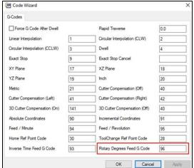
A Rotary Degrees/Min Feedrate option has been added to the Machine Parameters tab of the Machine Parameters dialog.
