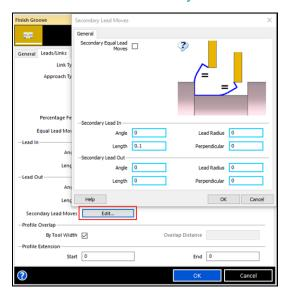
**Secondary Lead Moves** are now available on the Lead/Links tab of the Finish Groove cycle.
