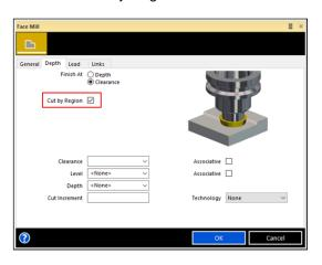
Because Face Milling can recognise the current stock, the cycle can be used to machine the top area of different bosses. However, previously, the cuts had no proper order and the tool could jump around between the different areas causing a lot of unnecessary moves.
