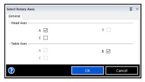
EDGECAM now supports a Horizontal Machine tool with A and C rotary axes in the head and a B axis Table.
