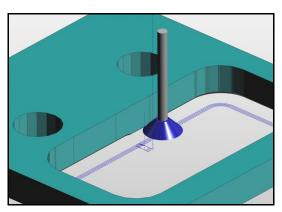
The Profiling Cycle has been enhanced to support **Multiple Passes** when using a Dovetail Cutter on Wireframe and solid edges. This option means that several passes can be taken to reduce cutting forces.
