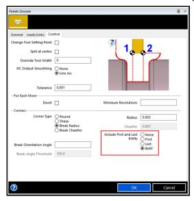
The Finish Groove cycle has been enhanced to allow the break corner to be applied to either the first, last or both sides of the groove.
