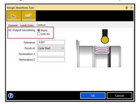
The Rough Waveform Turning cycle has been enhanced by adding a Smooth option to convert the line segments into fitted arcs. This can reduce the NC code by 75%.
