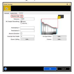
When Finish turning with a groove tool, and the only geometry selected is a single line parallel to the tool axis, the wrong side can be selected. We have introduced a new modifier to reverse the side if this situation is encountered.
