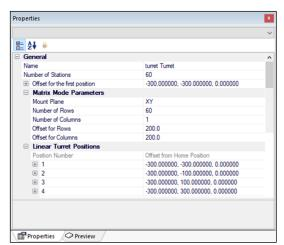
For linear mounted tools, EDGECAM supports a single line with a single pitch value. Some machine tools have variable pitch and also multiple axes to mount the tools.
