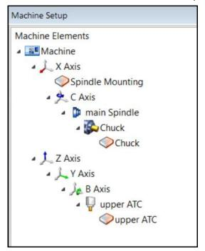
Normally a Turn/Mill CYB machine would have C in the spindle and XYZB axes in the Head.
